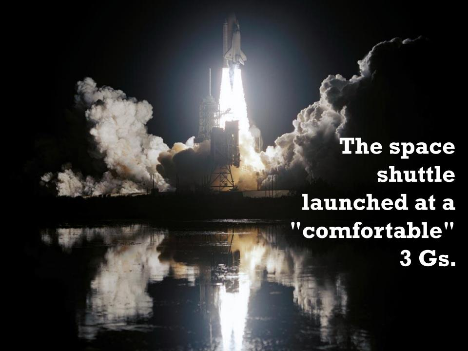
The space shuttle took off like a rocket but landed like a plane. *The* solid rocket boosters provided most of the push, or thrust, needed to launch the shuttle. The thin and long solid rocket boosters burned for about 2 minutes.
