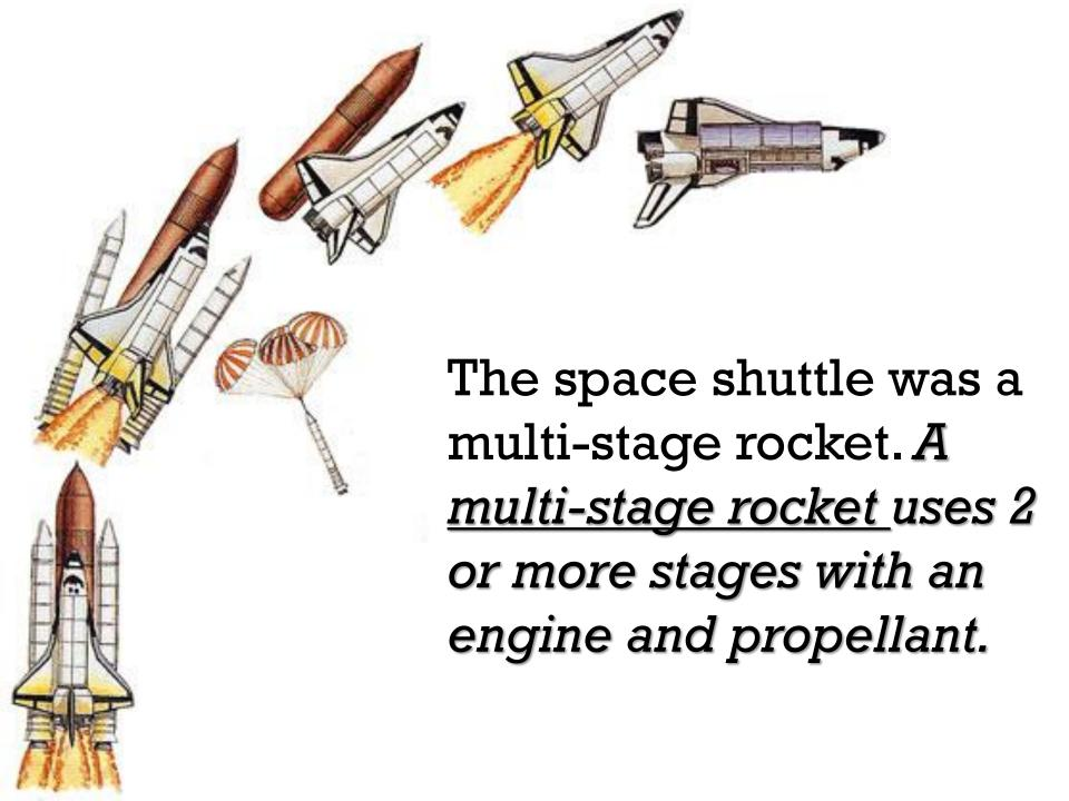
A rocket pushes forward when gases expelled from the rear of the rocket push it in the opposite direction.
