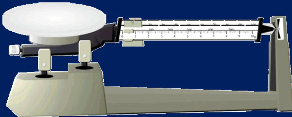
This measuring tool is called a triple beam balance.
