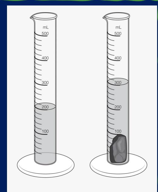
The cylinder measures 200 mL before the rock is added. After the rock has been dropped, the volume increases to 300 mL. The difference, 100 mL, is the volume of the rock.
