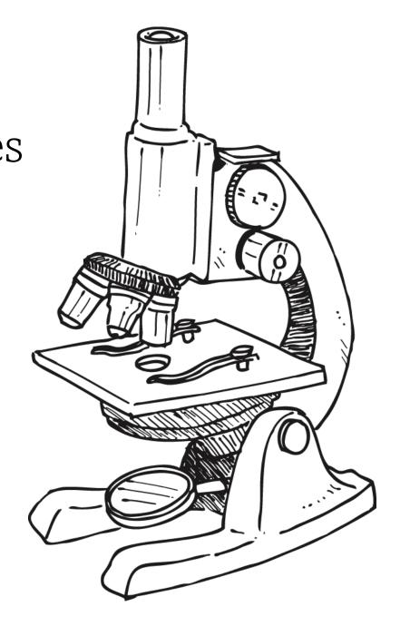
The eyepiece is the lens you look through to see the specimen. The lens is usually a 10x or 15x lens.
