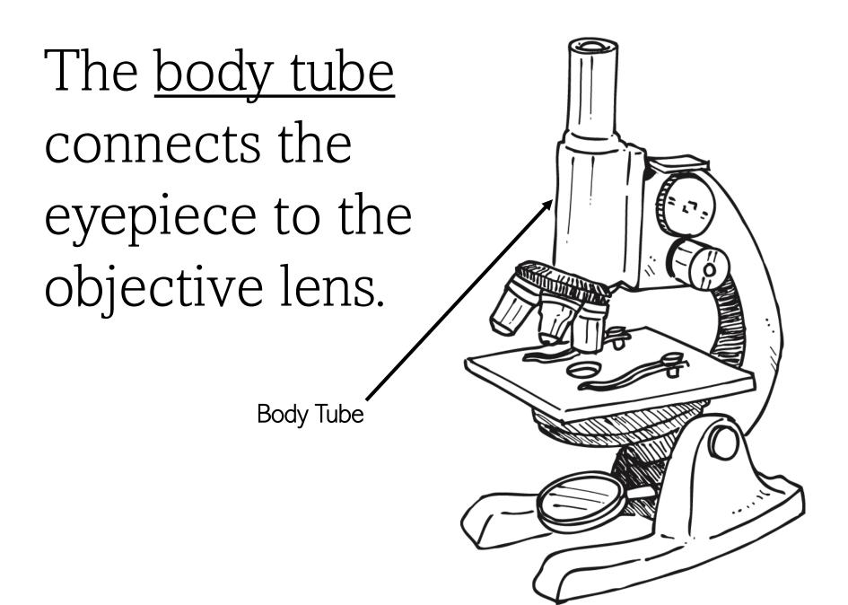
The <u>arm</u> supports the tube and connects it to the base. It is the part you hold to carry the microscope.
