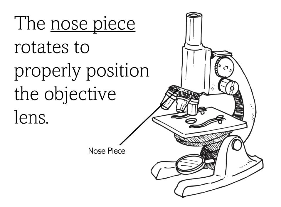
The objective lens magnifies the image of the specimen. A compound microscope has 3-5 objective lens that range in power from 4x to 100x.
