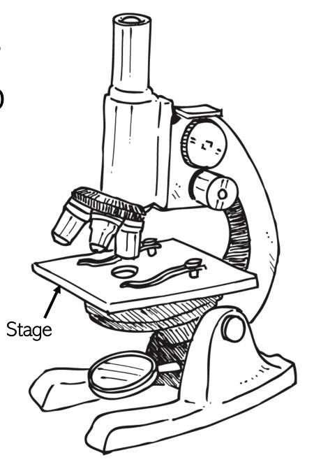
The stage clips hold the glass plate in place that holds the specimen being viewed.
